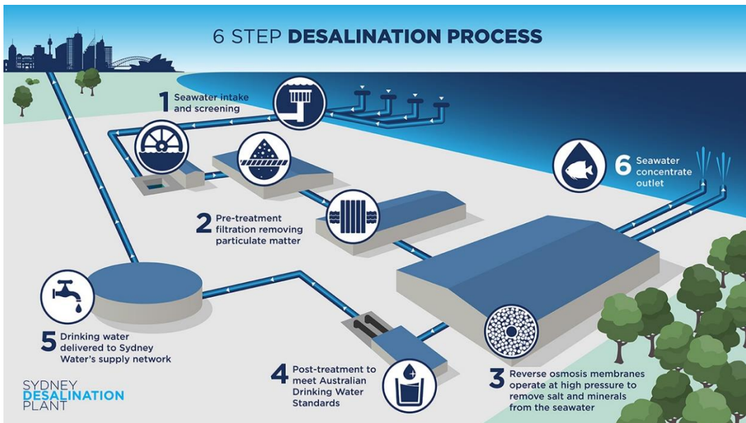
Figure 4: Schematic of Typical Seawater Reverse Osmosis System
