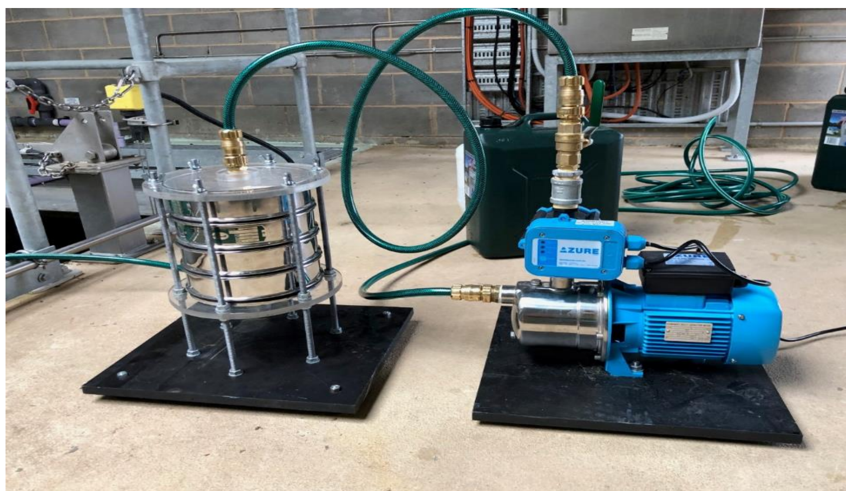
Fig.1. MP concentration and separation apparatus. Grab samples were pumped through four stainless steel filters of decreasing mesh size.
