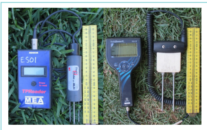
Figure 2: The Delta-T Theta Probe with MEA reader (left). The Campbell Scientific CS659 probe and HydroSense II reader (right).
