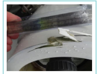
Photo 5: Major end impact damage
