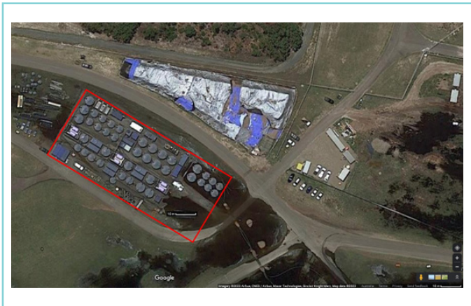
Image 2: Aerial shot of a conventional PFAS remediation at an Australian fire training facility. The visual shows the size of footprint, and thus difficulty, in treating water from such a facility and associated stormwater runoff with leaching PFAS. Photo: Google Maps
