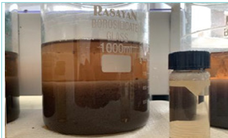
Figure 6: Red meat industry jar test results
