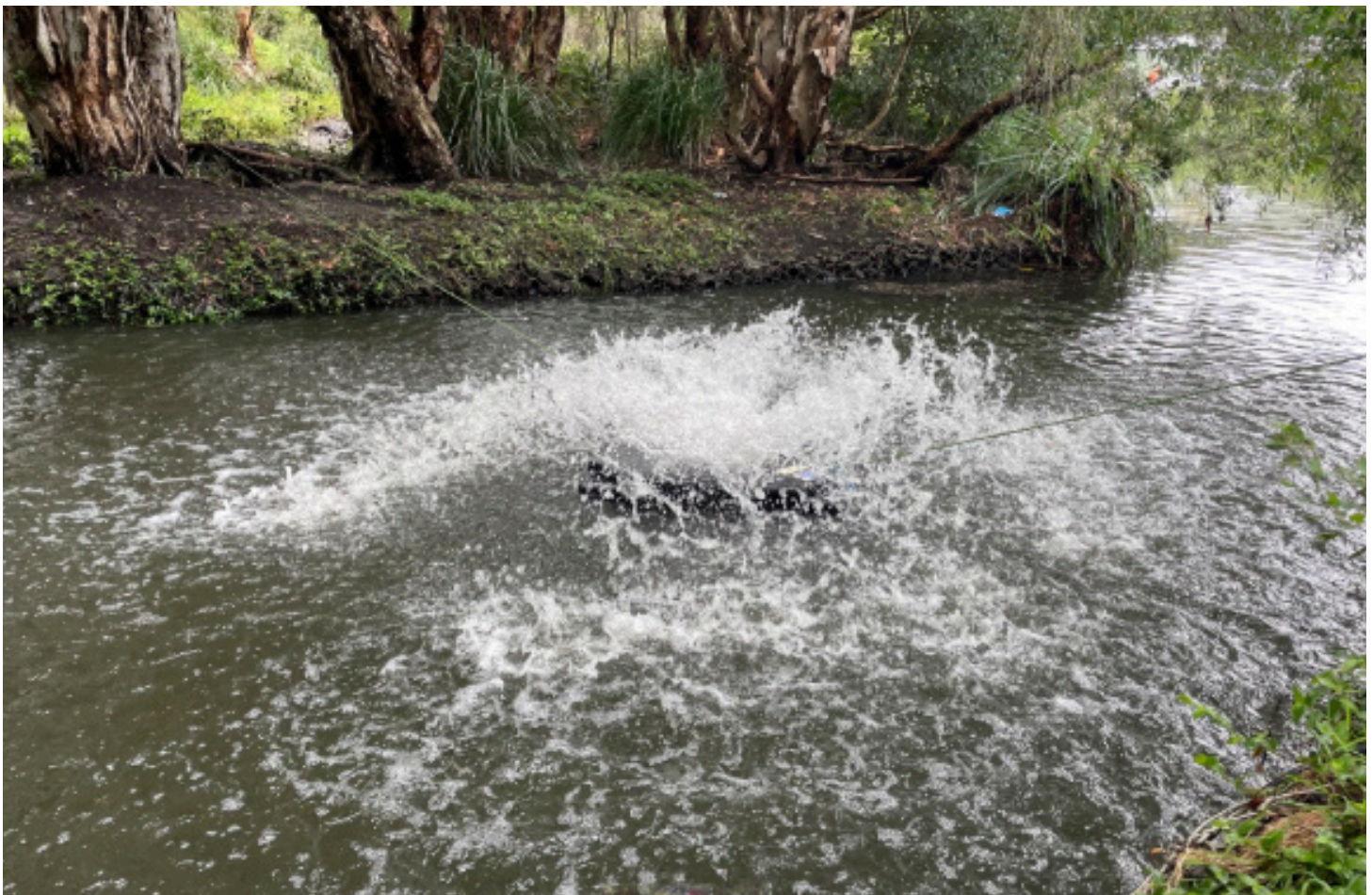
Figure 3: Surface aerator being trialled at Botany Wetlands Canal, Sydney
