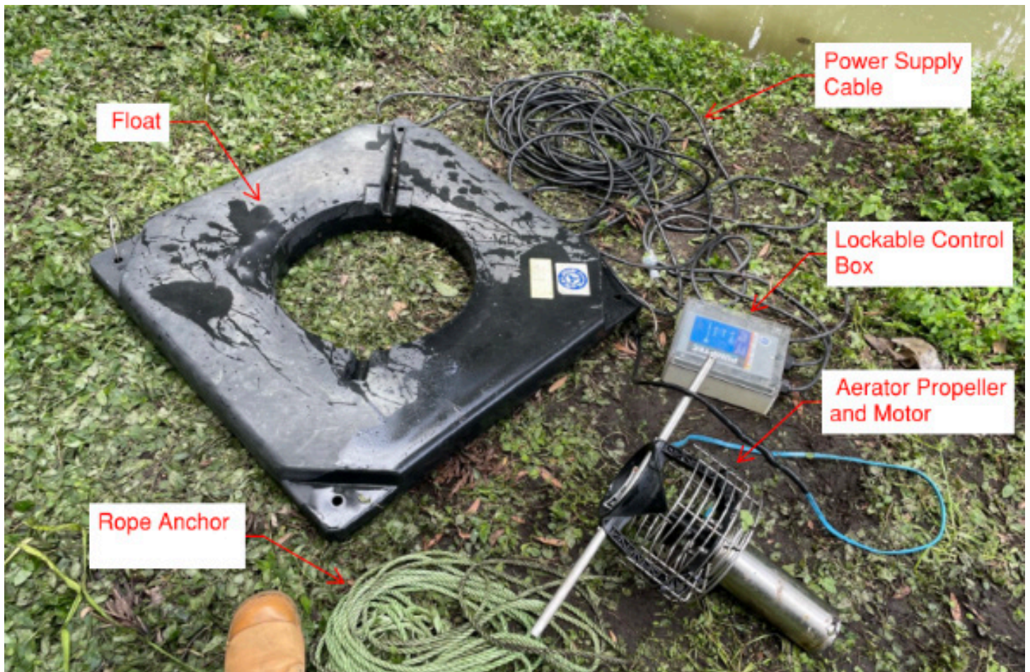
Figure 4: Surface aerator disassembled
