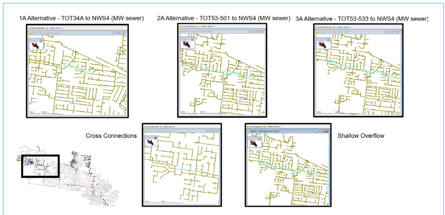
Figure 3 – The light blue pipelines are the alternatives introduced to the optimisation framework as possible interventions
