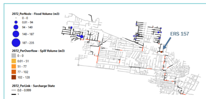
Figure 7 - Surcharge, flood and spill volumes | 2072. Scenario with 2072 projection presents several flood areas and intensification of spill volume at ERS157.
