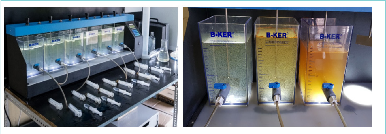
Figure 2: Jar tests and evaluation of floc characteristics
