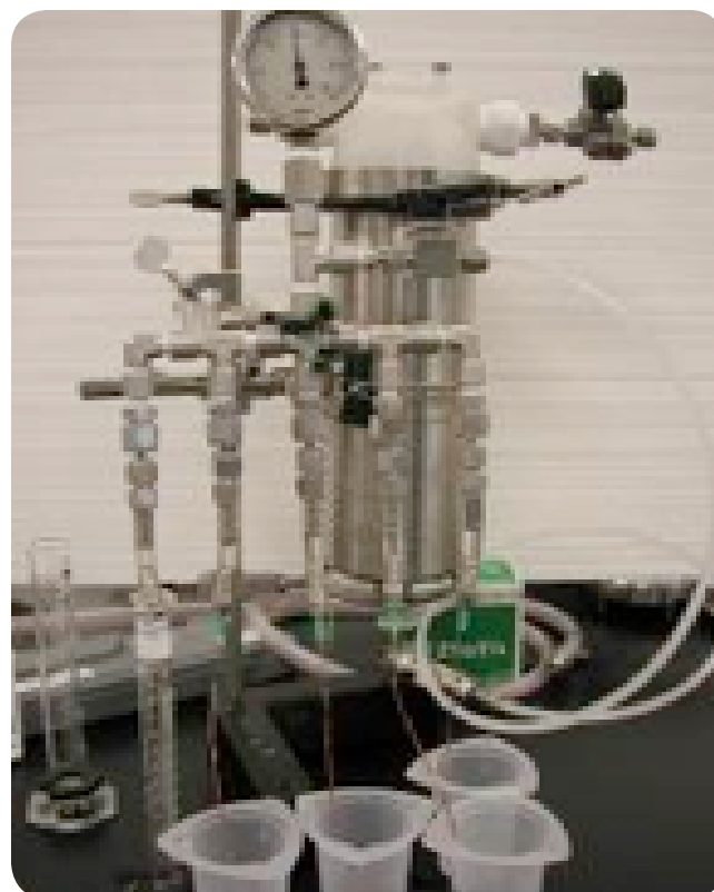
Figure 4. The bench-top testing stand for cleaning study of hollow fiber membrane samples
